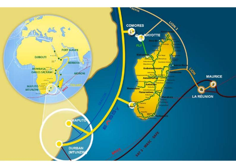
Telma has deployed wholesale solutions in Madagascar. This portfolio comprises an international connection via the **submarine cable, EASSy** (which Telma is a major investor in); a national transmission via the National Backbone in optical fiber; and network access (FO/ASDL/SDSL/WLL).
